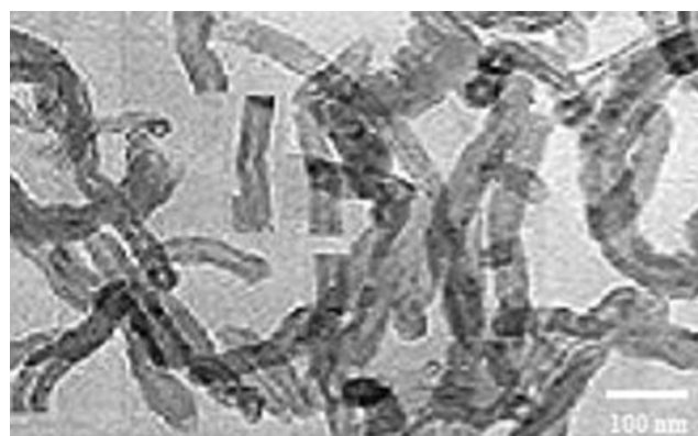
Fig. 2 TEM image of FUCO-MWCNTs.
